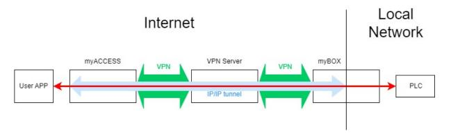
Communication schema: the secure VPN tunnel is created between user PC and VPN server and between VPN server and myBOX device.
